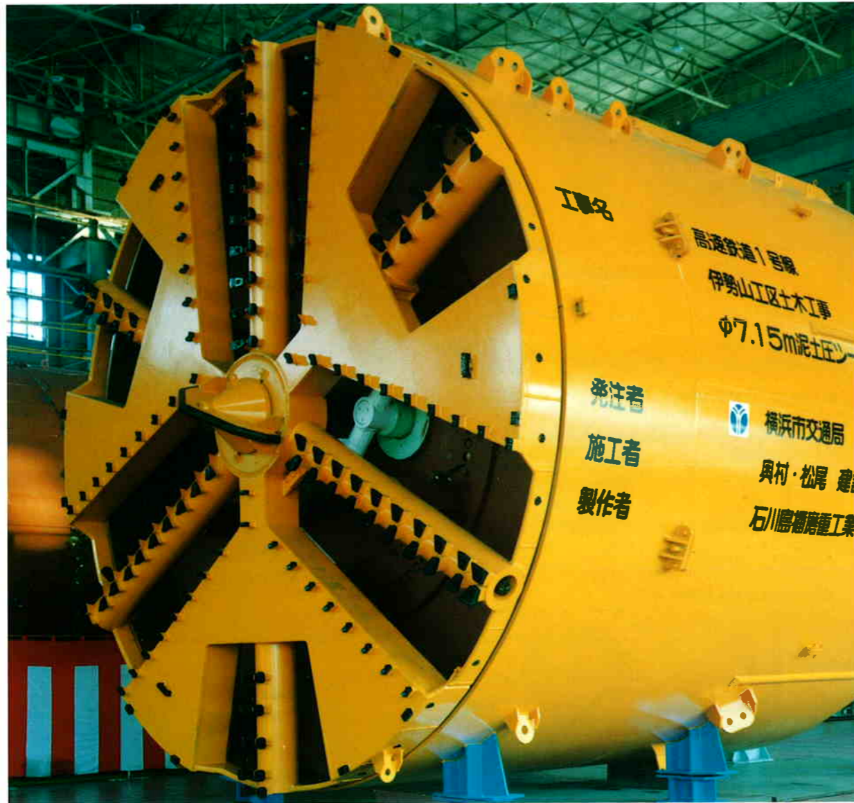
7.15 mφ mud injection type earth pressure balanced shield machine
