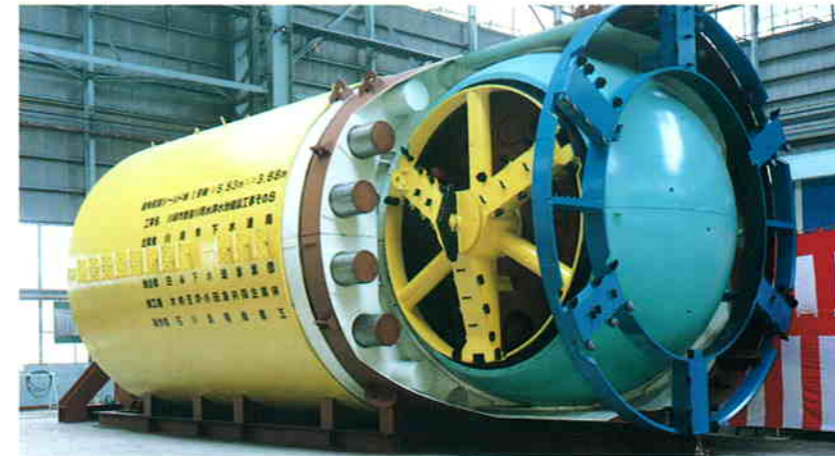
5.53 × 3.68 mφ right angle shield machine
