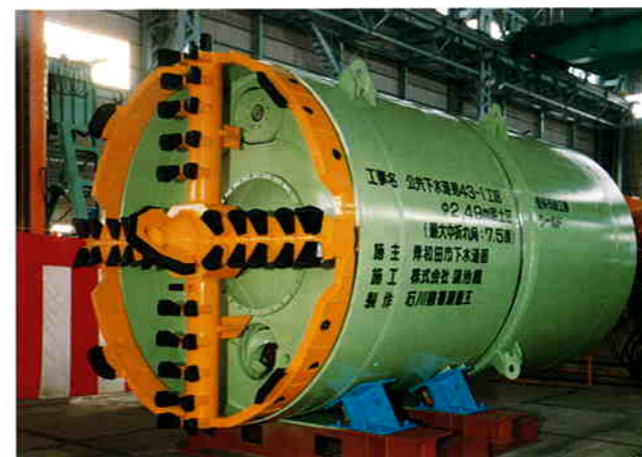
2.49 mφ muddy soil pressure balanced shield machine
