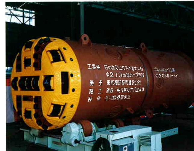
2.13 mφ muddy soil pressure balanced shield machine for bedrock and gravel
