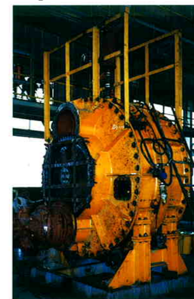
Cutter seal performance test
