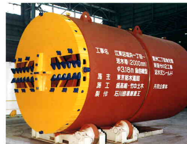
3.18 mφ slurry shield machine
