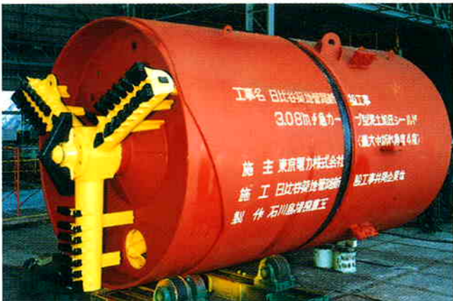
3.08 mφ muddy soil pressure balanced shield machine
