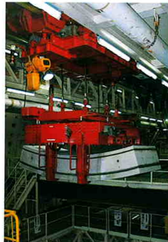
Segment carrying hoist
