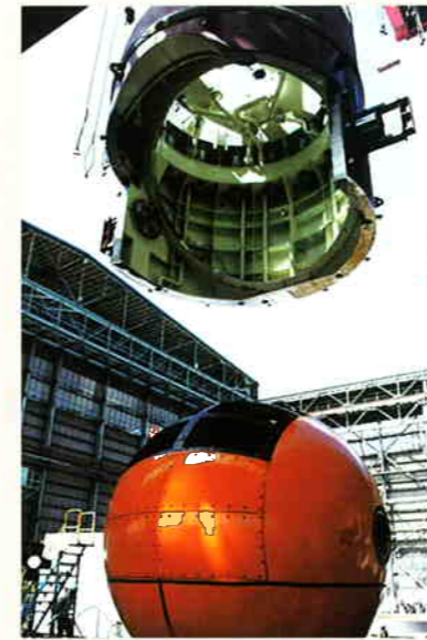
Rotating shield machine assembly
