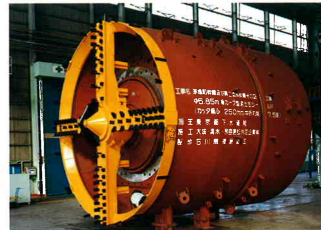
5.85 mφ cutter face eccentric type muddy soil pressure balanced shield machine
