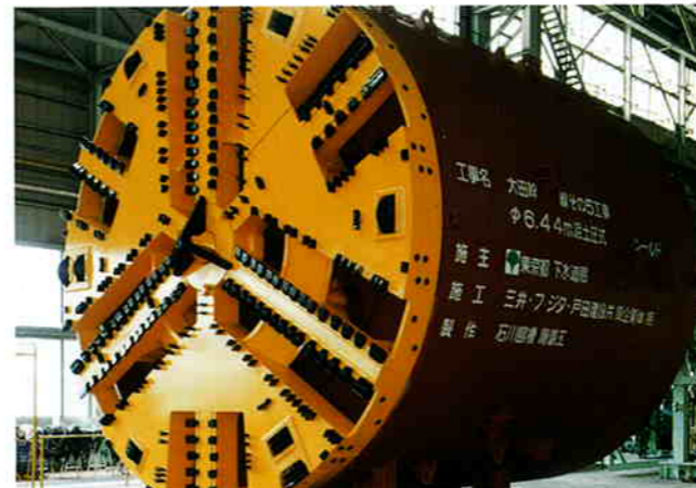
6.44 mφ muddy soil pressure balanced shield machine
