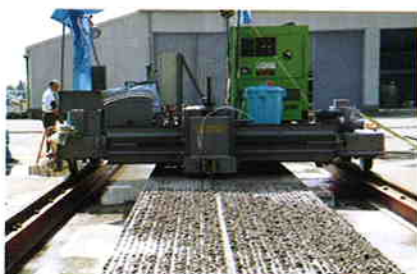
Cutter bit wear test
