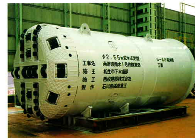
2.55 mφ slurry shield machine for bedrock and gravel
