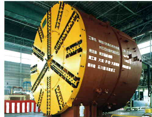
10.5 mφ slurry shield machine
