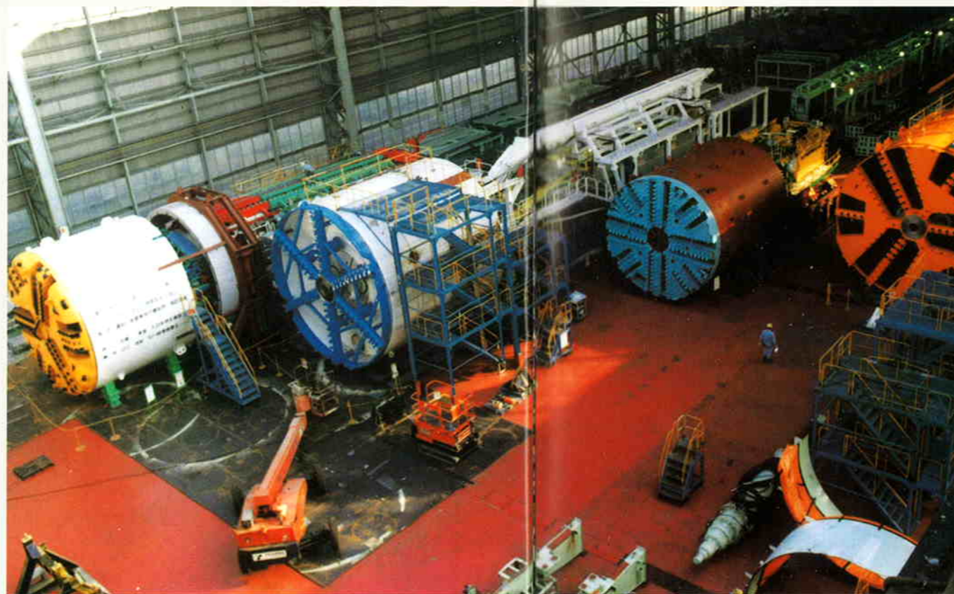
7.25 m \phi slurry shield machine being lifted.
