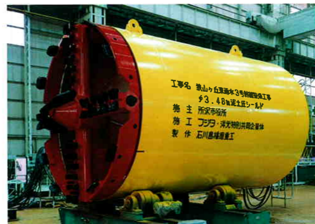
3.48 mφ muddy soil pressure balanced shield machine
