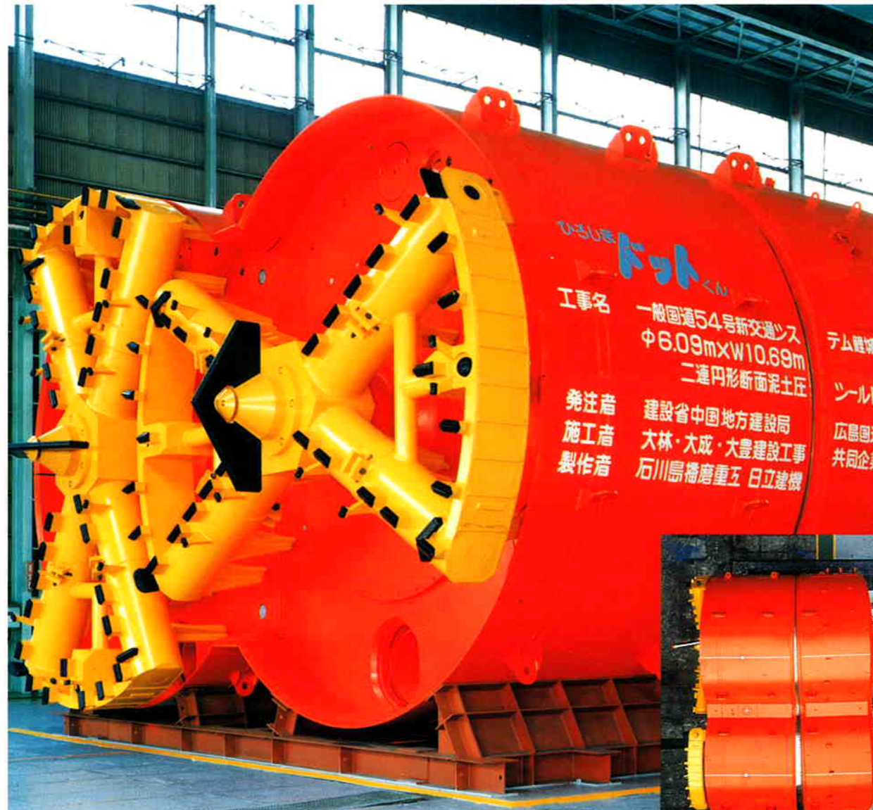
6.09 mφ × 10.69 mW DOT shield machine
