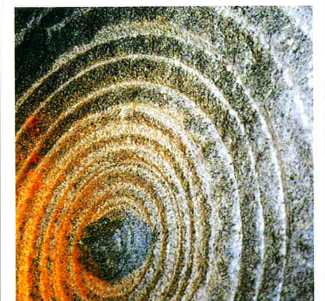
Face of bedrock cut with a roller cutter.
