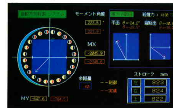
Automatic shield machine alignment control system
